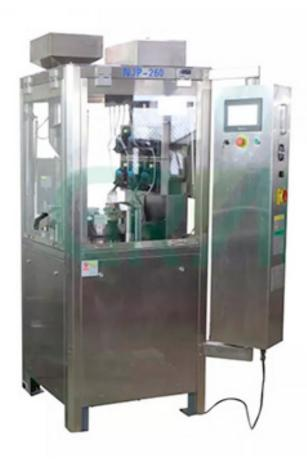
The maximum production capacity of this machine can reach 260 capsules per minute. Standard and serial production: the interchangeability of manufacturing parts can reach above 99%; each spare part has its own regular code; while changing the mould, all the parts are fixed by the location hole with high precise; it's very efficient to change the moulds, easy to operate and clean the machine.
