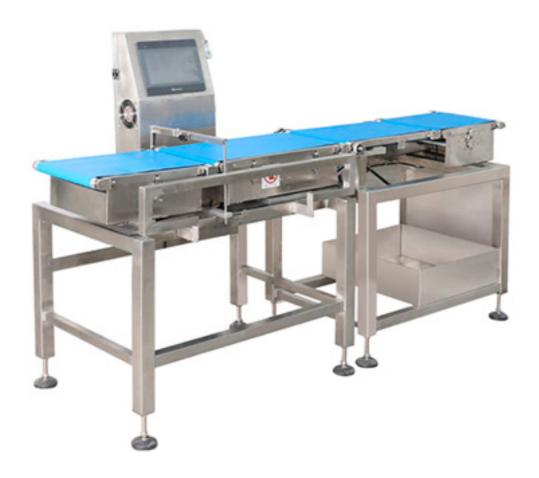
ZT Series checkweighers can handle various pack types, including bags, trays and cartons and are suitable for most production environments. Innovative modular design makes the checkweigher easy to clean minimizing downtime. Accurate and reliable, it utilize the latest weighing technology and offer various reject devices best suited to the line configuration.
