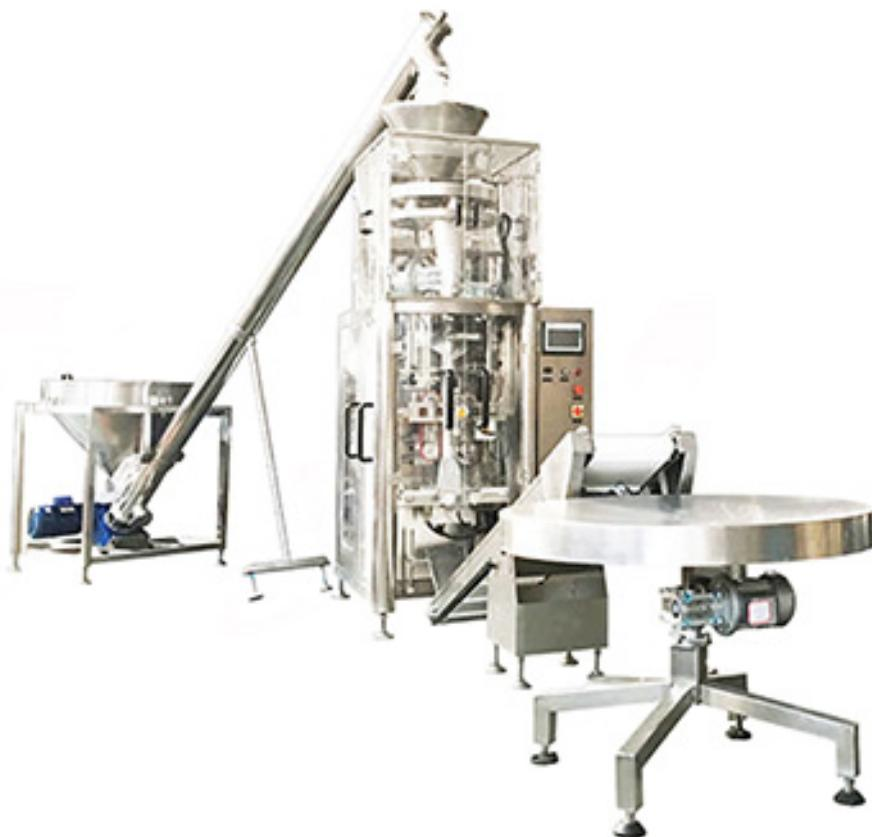
It is suitable for weighing packing dry food with irregular shapes and requiring high measuring accuracy, such as: rice, seeds, bean, grain, pet food, salt, nut, etc non-fragile and granular products.
