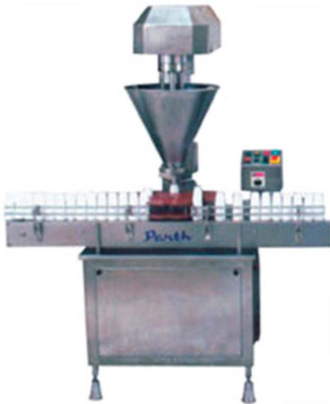
Vitro Pharma Machine provides Dry Powder Filling Machine which is specially designed for the pharmaceutical industry to fill powder in the Vial. In this Dry Powder Filling model, dry injection powder filling & stoppering machine is carried out on a single frame structure.
