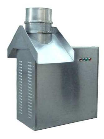
The machine can make necessary granule from the stirred raw material, it also can crush abolished slice and dry piece crowd it into granule. Especially, it is very suitable for raw material of higher viscidity.
