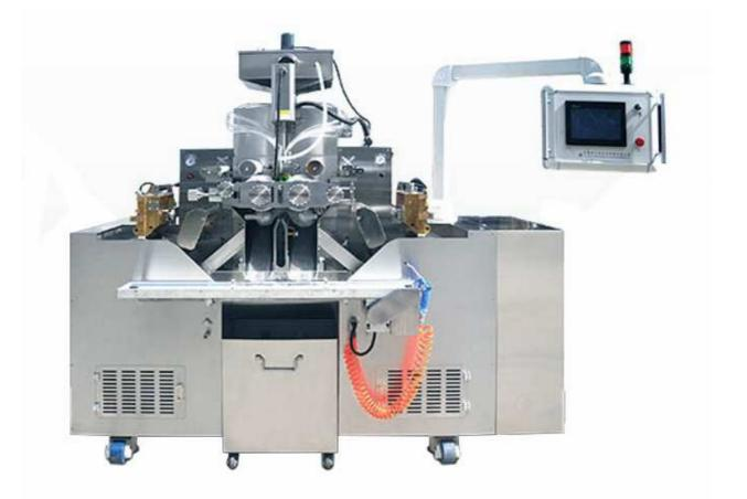
RJWJ-250 soft capsulation production line is of large scale production equipment. The single unit annual production capacity is 400,000,000 capsules. Adopts international advanced control technology, precisely design precisely producing, it is the dependable tool for the production of high quality soft capsules.
