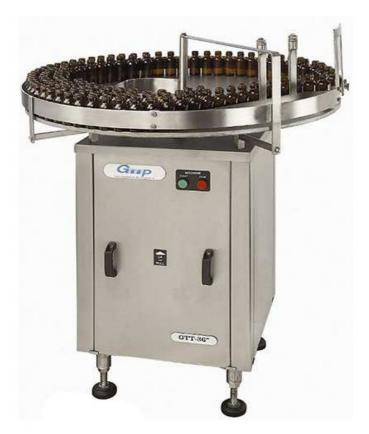
Stainless steel scrambler & Un-scrambler, which is familiar as turn table. This is built on SS Square frame, solid guide rail & reduction gear box for jerk less & noiseless performance. Turntable is useful to ensure total synchronization, uniform flow of container and to take a turn at 90 degree to suit different machine and purpose in automatic liquid line.
