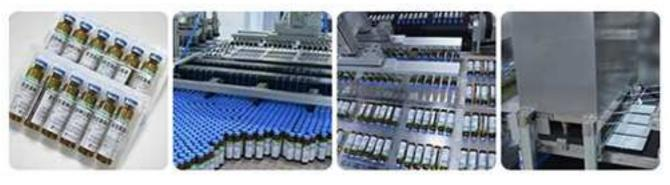
Colamark B200 is a thermal formed blister packaging machine which automatically forms blisters, inserts materials, and die cuts in one process. Designed for the packaging of small containers, ampoules, oral drink bottles, syringes for the pharmaceutical industry, at up to 600 pieces per minute.
