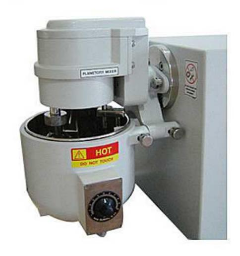
Planetary Mixer Heating Jacketed mixer is designed to be used as a mixing for pastes, ointments & creams in water jacketed kettle. It can also be used for wet powders. This mixer is provided with a mixing paddle and Teflon scrapper, which is shaped in such manner so that there is minimum clearance with the mixing kettle. Temperatures of kettle can be adjusted by the help of thermostat knob. The kettle is also easily removable.
