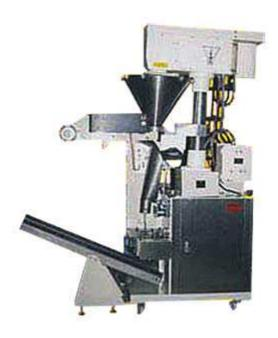
Suited for filling food, pharmaceutical chemicals, and agricultural chemicals. 35 - 65 angle of repose or particle allowed break, and other non-free flowing powders.
