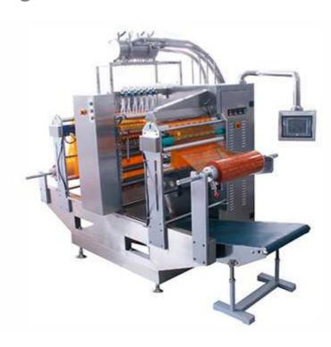
As shown in the picture, the packing machine is used for packing liquid materials such as soy sauce, vinegar, wine, medicine, chemical agents and so on, providing measuring and automatic packing into sachets. It is used in the medicine, food, and daily chemical industries. Note: This range of equipment is designed with filling capacity between 5 and 100ml. It is not suitable for occasions with filling volume exceeding 100ml.
