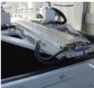
Electronic-impulse gusset-type sealing system providing watertight bales
