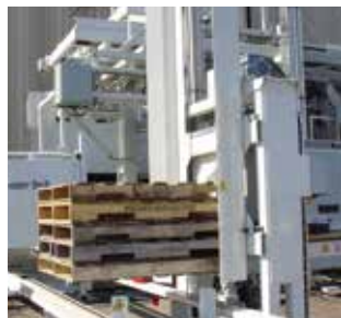
Automatic palletizing system including pallet dispenser and safety fences available
