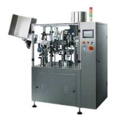
Auto Plastic Tube Filling and Sealing Machine
