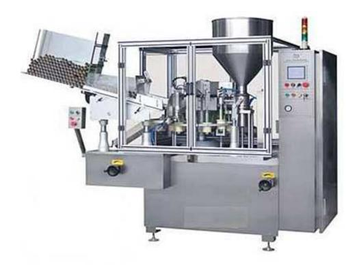
Automatic Paste Tube Filling, sealing and coding Machine ATFM-50 R We specialize in manufacturing Automatic Paste Filling Machine which is suitable to fill any type of viscous paste, creams, shampoo, food paste pickles, chutney, wax, petroleum jelly, ointment, tooth paste, honey, paints, adhesives etc. in bottles, jars, cans, stand-up pouches, tubes etc.
