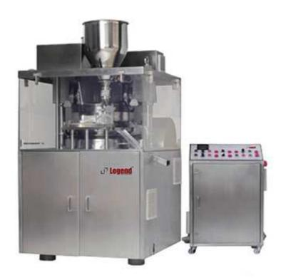
Legend Prima Press Double Rotary Tablet Compression machine (GMP Model) with maximum output up to 270000 Tabs/hr is available in D" ,B" & BB" tooling . It comes with special features of AC VFD drive, electromagnetic clutch & Auto Lubrication system.
