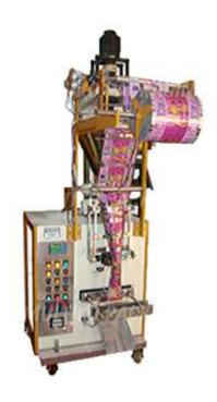
The MK-204 is a semi pneumatic vertical form fill seal packaging (VFFS) machine designed to package various sticky and non-sticky powder products. This vertical packaging machine uses auger dosing system to produce center sealed and 3 side sealed pouches / bags.
