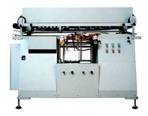
It is applied for the tin can's labeling. It adopts horizontal labeling when the can is rolling with high speed. The glue is only spreader on both ends of the sticker, and the head is with hot glue, and the tail is with cold glue. The sticker can be pressed steady, and no can no glue. And the labeling speed can be adjusted by the transducer. It is the ideal equipment of can labeling.
