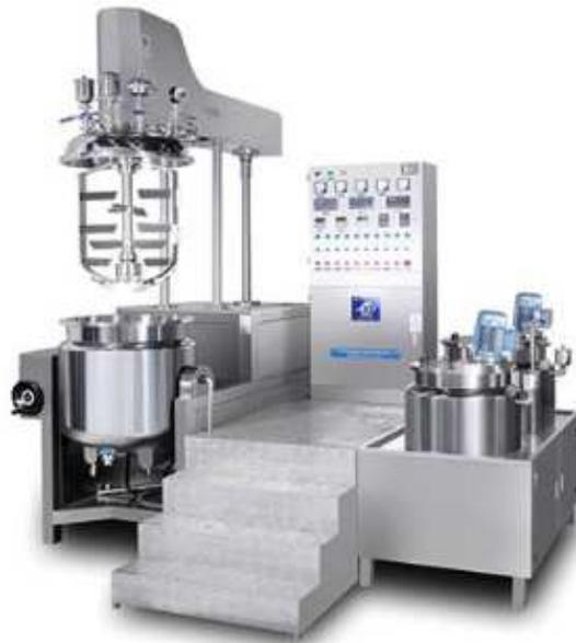
RHJ-C Vacuum emulsifying mixer (Upper homogenizer type), this series machine adopt two mixing speed on one shaft to make high viscosity product more smooth, homogenizer make it upper in the perfect position to reach best emulsion function, homogenizer speed is 0-3600RPM, hydraulic lifting system for product outlet and machine clean and maintenance more convenience.
