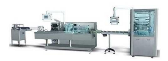
This machine is suitable for automatic feeding bottle (round, aquare bottle) into carton (either for blister or bottle). On line bottle unscranble and feeding, leaflet fold (1-4 folds) and feeding, carton opening and forming, products and leaflet pushing into carton, printing batch number, sealing carton with tuck-in or hot melt glue device. Automatically reject lacking of leaflet or product and finished product out.
