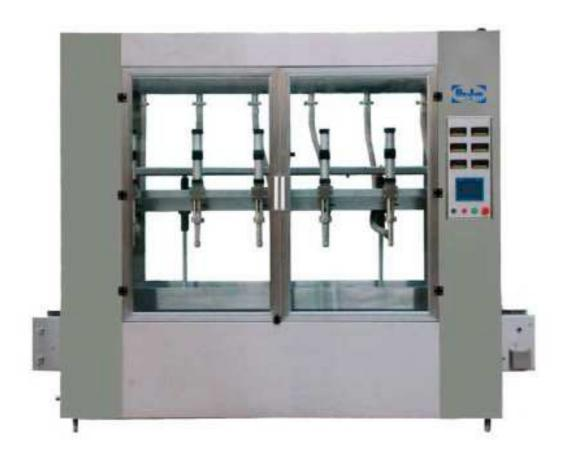
This machine is making up of the scale (with roller), chain-driven drum in and out structure, fast and slow filling (with dive function), material tank, weight control meter and PLC control unit. This filling machine can do the auto filling of different materials. It has the dive function can eliminates the splash and foaming can.
