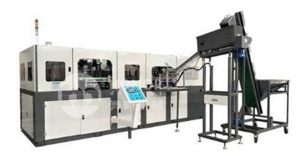
Bottle blowing machine is a kind of equipment which can make plastic granules into hollow containers by blow molding process. It is mainly used in beverage and food industry.
