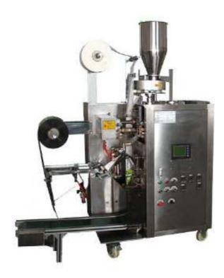
The packaging pouches with drawing line and tag. The process of bag making, measuring, filling, sealing, cutting and counting can be done automatically.
