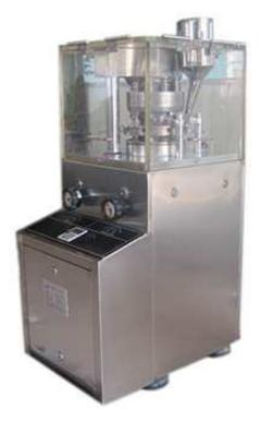
Rotary tablet press is a mechanical device that compresses powder into tablets of uniform size and weight. This machine can be used to produce tablets of a wide variety of materials, including pharmaceuticals, cleaning products, and cosmetics. To form a tablet, the granulated material must be metered into a cavity formed by two punches and a die, and then the punches must be pressed together with great force to fuse the material together.
