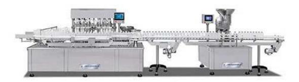
This infusion bottle filling line contains processing of feeding, filling, plugging, capping and labeling. The line meets GMP requirement with high efficiency and anti-leaking function. Easy operation with PLC controlled and adjustable parameters in touch screen. Each machine can be used stand-alone, also can be used for filling line. The filling line is widely used in pharmaceutical, chemical, veterinary drug industries.
