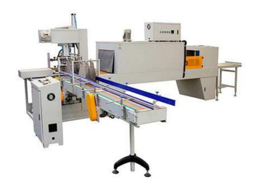
This machine is used in the combination package of mineral water, beverage, beer, liquor, infusion bottle and so on. The packing is not needed.
