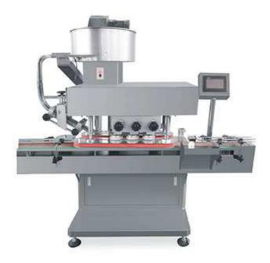
Equipped with three pairs of friction wheels, self-adjust tightness, helpful the caps surface. Wide applicability, it is simple and convenient if change bottles and caps, just adjust some components. Equipped with human-computer interface and PLC control system, Ensure more stable operation and easier handling. Self-diagnose errors and stop working to make alarm at errors and missing bottles, caps. The bottle with twisted cap, anti-cap and without aluminum foil will be removed.
