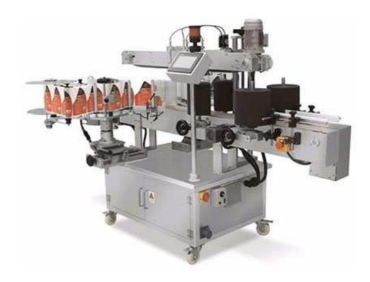
Automatic Labelling machine Put the labels roll on the roll holder, the machine can do put the labels on the containers, and then do labelling automatically. Automatic labelling machine can do labelling for round bottles and also can do two sides labelling for flat bottles or square bottles.
