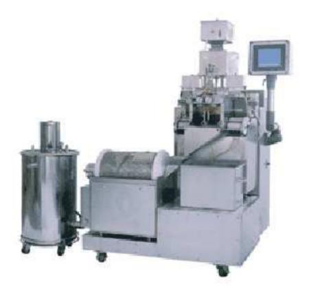
Model RGY×15F Soft Gel encapsulation machine is a new model developed by us in 2001. The machine consolidated the features and production technology of the soft gels, it is designed fully in compliance with GMP, using the newest technologies and materials. The power needed for the machine is 220V, in one phase. It is mainly dedicated to laboratories and pharmaceutical research institutions for development or pilot production of soft gel products.
