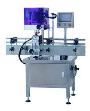
The automatic capping machine is controlled by touch screen, parameter can be set on touch screen easily.
