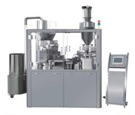
NJP-5500C Automatic Capsule Filling Machine adopts butterfly valve-type powder feeding, and is very suitable for drug powder with poor liquidity, including Chinese herbal medicine and Chinese patent drug, due to that its vibration unit equipped will force the powder to run down, which has solved problem of failing to feed in powder that often happens in the traditional screw feeding device because of the poor liquidity of powder.
