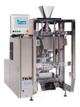
This standard but very functional vertical form-fill-seal machine was created based on TAM's pursuit of exceptional film feeding and sealing performance. When the machine is running, operators can view the operating status and monitor the temperature, pressure, and closure location on the sealing bar.
