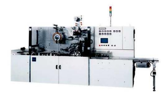
The high speed film overwrapping machine model can wrap products at maximum 200 ppm. Automatic feeding device and failure elimination device are equipped as standard specification. Servo-driven film feeding and film transfer by suction belt allow stable operation. With combination of option devices W3701 can corresponds to the total packaging line system.
