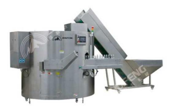
The machine is used to sort the polyester bottles, and the scattered bottles are sent to the bottle unscrambler through the hoist. By the thrust of the turntable, the bottle enters the bottle slot and locates itself. Through the action of the turning device and the air flow, the bottle mouth is upward. And through the wind-feeding bottle system output into the next process.
