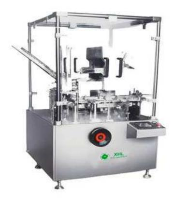
This product is a modified and improved new model in combination with the domestic and abroad advanced technology. It is a high-tech product that integrates the machine, electricity, air and light. electricity, gas and light. It is widely applied to the box packaging of aluminum-plastic, medicine bottle, cosmetic products, Poker cards, electronic products and other daily chemical products, or similar particles.
