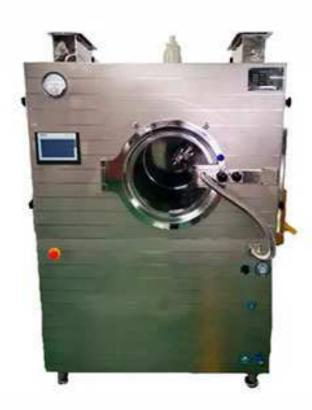
The efficient coating machine consists of major machine, slurry spraying system, hot-air cabinet, exhaust cabinet, atomizing device and computer programming control system. It can be widely used for coating various tablets, pills and sweets with organic film, water-soluble film and sugar film etc.
