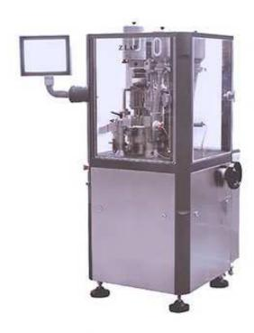
Automatic Capsule Filling Machine processes the products for optimal productivity up to 12,000 capsules per hour, featuring low-maintenance operation, minimal downtime, and overall dependable production.
