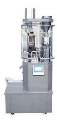
It adopts hole plug type filling, batch-type running and frequency control. It is suitable for the whole capsule filling process: capsule feeding, separating, filling (waste capsule rejecting), closing, perfect capsule outputting, for powder and micro pill capsule.
