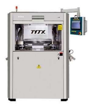
The diameter of the pre-pressure whell and the main pressure are the same, which can reach bigger pre-pressure value, the max pressure, pre-pressure both can reach 100KN, bigger pre-pressure can guarantee the tablet exhaust well before the moulding on line, it will be reduce the break of the tablet, meantime increasing the speed.
