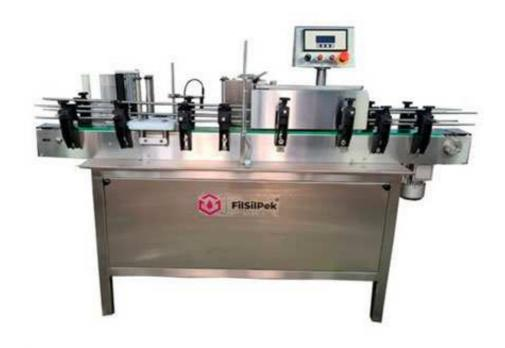
The Automatic Vertical Sticker Labelling Machine is one of the most users friendly. The machine is used for full/partial wrap around labeling on different size of round containers. The automatic model is equipped with roller spacing device resulting in a simple operation with "No change parts required".
