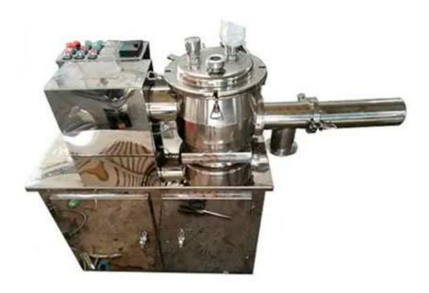
It is suitable for pharmaceutical, foodstuff, chemicals industry and so on. The granule is made from power to damp granule in which the adhesive should be injected in it.
