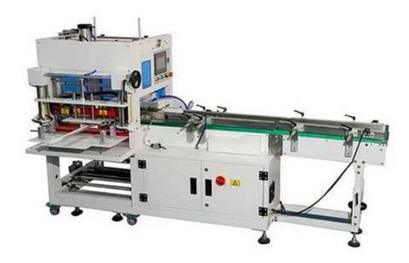
ZF-X500T cylinder packing machine is used for multi roll tape cylinder packaging, the packaging effect is very beautiful. It can also be connected with automatic slitting machine to form automatic product packaging production line and improve production efficiency.
