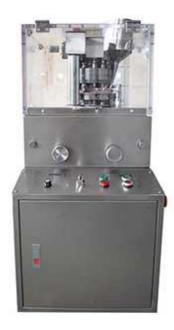
ZP10, ZP12 Rotary tablet press is a new generation product by our factory, and this machine is a single roller continuous automatic tablet press for pressing various kinds of different shape tablets and plain tablets, such as round tablet, irregular tablet and carved tablet etc.
