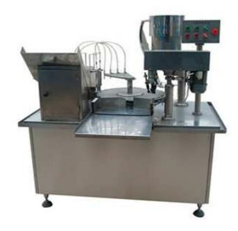
This machine is the main filling & sealing equipment of the Yilagai (or aluminum-plastic cover) production line, which is mainly applied in the filling and sealing of 5 - 30 ml bottles.
