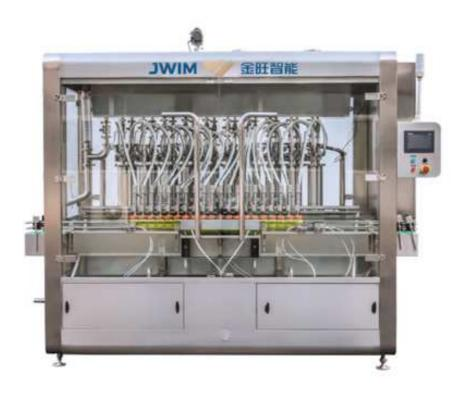
Automatic linear piston filling machines are extremely flexible piston fillers capable of filling accurately and rapidly a wide variety of products from low viscosity liquids to high viscosity paste or cream with or without chunks or particulates. Widely used in the Chemical industry(e.g., grease filling machine, lubricant filling machine, etc); agrochemical industry(e.g EC filling machine, SC filling machine, etc).
