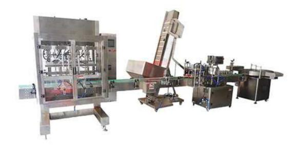
Our automatic linear structure shampoo filling machine adopts the principle of plunger quantitative filling, bottle feeding, positioning and filling, the bottle is automatically controlled by PLC, which conforms to the GMP standard. It is suitable for liquid filling of medicine, food, daily chemical, pesticide, fine chemical industry, etc.
