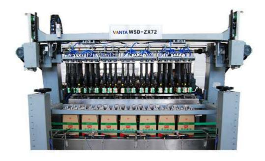
Carton Packer is a piece of packaging equipment which packing containers into plastic or cardboard cartons in certain arrangement. It satisfies containers in round, oval, square, canned and other special shapes and has been widely used in packaging line of beer, beverage and food industries.
