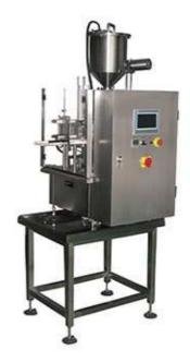
The rotary cup filling and sealing machine is specially offered for packaging liquid with pre-made plastic cup, paper cup, and paper-plastic cup, singly. The rotary stepping type filling and sealing equipment is suitable for packing liquid or semi-viscous material, for example, yoghourt, milk beverage, soya-bean milk, fruit juice, jelly, ice cream, seasoning, and everyday chemical.
