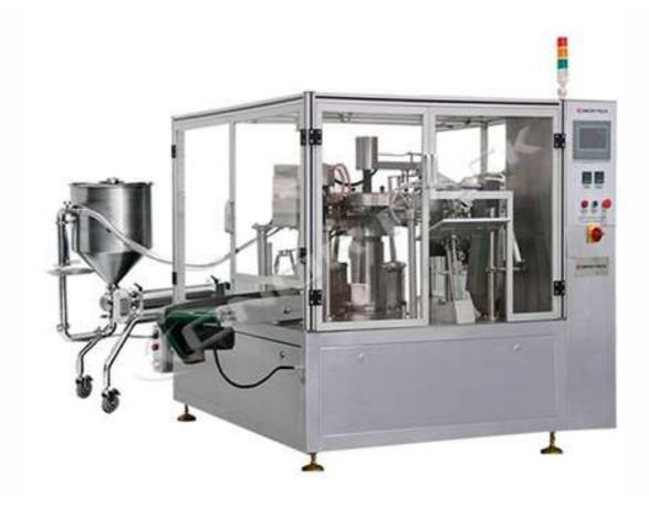
Equipped with piston filler as the dosing system, it is widely applicator to packing liquid and paste, such as detergent, softener, shampoo, shower gel, milk, water, juice, soybean sauce, oil, ketchup, mayonnaise and so on.
