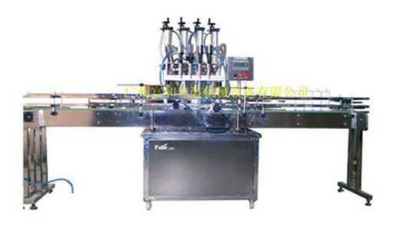
FH-4G series piston type, filling and sealing all-in-one machine, the structure is compact and high degree of automation, so it can have mass assembly line work in a small space. The filling system all adopts import pneumatic element FEST0, which the machine has powerful motive power and high reliability in filling different high viscosity liquid products. In the machine all the contact surface and corner piece with liquid, the roughness reach 0.5um, correspond GMP standard.
