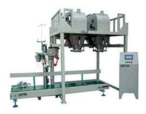
This machine is intended for use in granular quantitative packaging. It uses a free-fall delivery system, fast and precise valves make the material feeding process frequent and stable. With an internal weighing bin, increase packaging volume. The final solution has a compact structure: free space, low power dissipation, good and laconic appearance.
